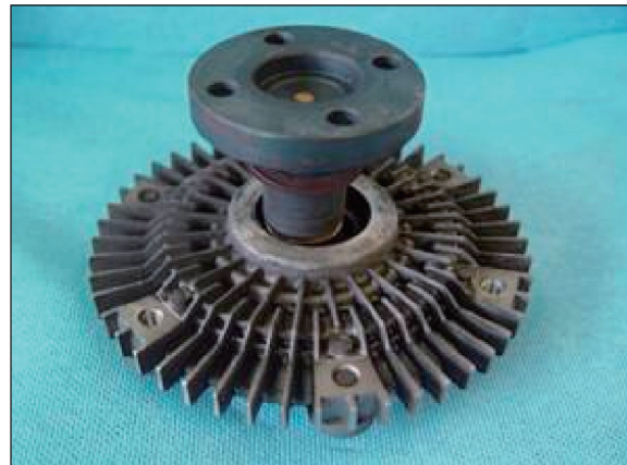
Fan clutch bearing blocked → breakage
